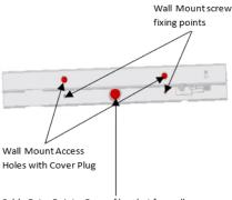
Cable Entry Point – Rear of bracket for wall mount, 20mm diameter, located in centre of
